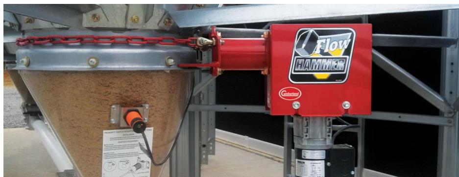
Figure 2: Cumberland Inc. Flow Hammer and proximity sensor mounted to feed bin collar (Cumberland)
