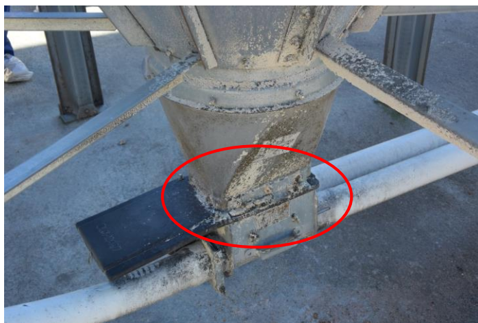
Figure 5: Location of transition piece to be adapted in Alternative 1
