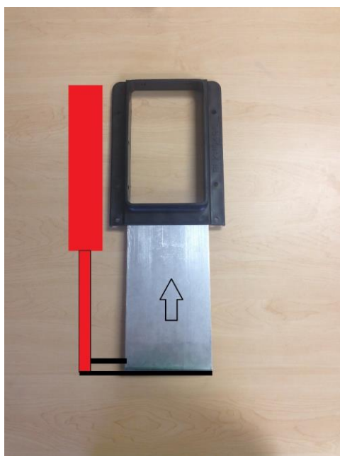
Figure 6: Alternative 1- side mounted linear actuator system
